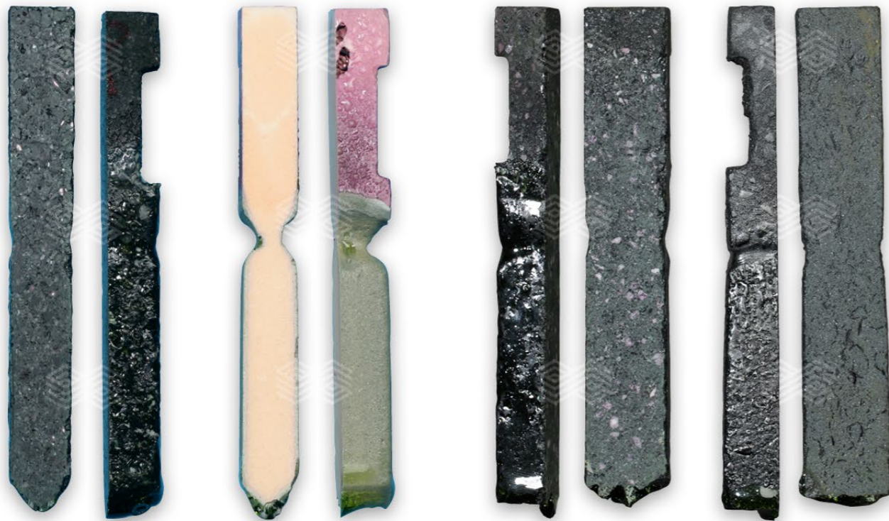
SUPRAL RK5OS与电熔AZS的耐腐蚀性对比 / Corrosion of SUPRAL RK5OS compared to fused cast AZS
