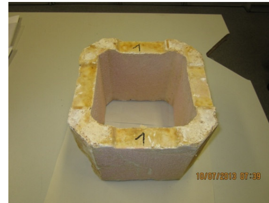
Rubinal EZ: no gluing and no corrosion after 7 years
