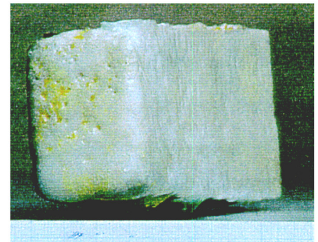
Rubinal EZ: no gluing and no corrosion after 7 years
