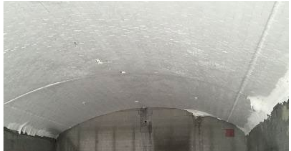
Stella GNL after 10years campaign in an oxyfuel furnace
